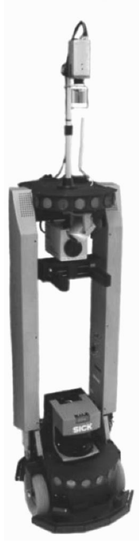
Figure 9-3. ActivMedia Peoplebot. It is equipped with a SICK LMS 200 laser scanner and panoramic camera (NetVision360 from Remote Reality).
