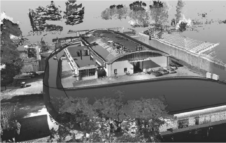
Figure 10-6. Sample model from a vehicle-mounted scanner. (See also Plate 32 in the Colour Plate Section)
