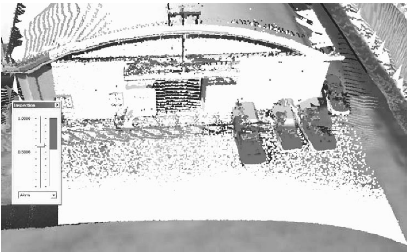
Figure 10-20. Results of scene change detection with alarm coloring (white = 0-0.5m diff, red >0.5 m diff). (See also Plate 37 in the Colour Plate Section)
