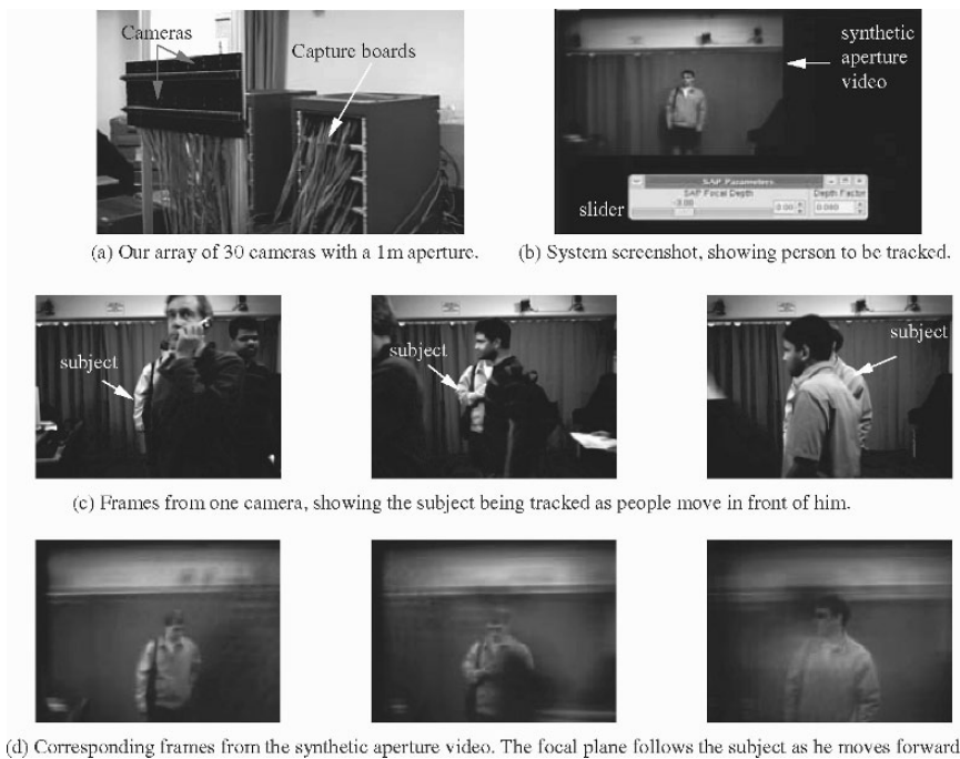
Figure 7-5. Real-time synthetic aperture video, used to track a person moving through a crowd of people.
