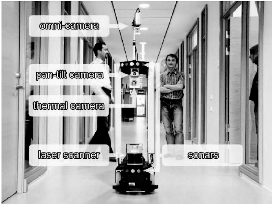
Figure 9-1. Robotic platform for security guard with sensors marked. The laser range scanner and the omni-directional camera are used to build a 3D model of the robot's operation environment.
