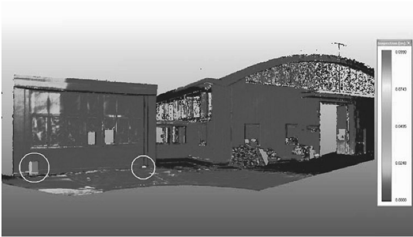
Figure 10-15. Result of change detection of an outside environment. (See also Plate 35 in the Colour Plate Section)
