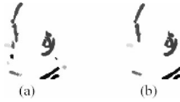
Figure 6-5. (a) Labeled image (12 components). (b) Labeled image after removing smaller components (6 components). (See also Plate 22 in the Colour Plate Section)
