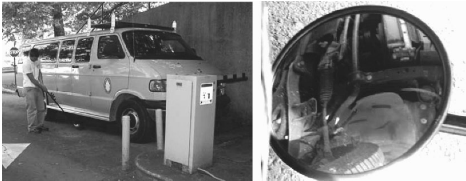
Figure 11-1. The traditional method for inspecting a vehicle undercarriage is to use a mirror attached to the end of stick. This mirror-on-a-stick approach enables security personnel to search wheel wells and other vehicle cavities. On the right, we show a picture of the scene the inspection personnel views on the mirror.
