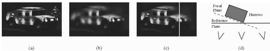
Figure 7-3. User-driven change of focus. (a) An image from a light field showing a toy humvee at an angle to the plane of cameras. (b) Synthetically focused image on reference plane. Note that the left side of the humvee is out of focus, since it is not on the reference plane. (c) If we rotate the focal plane about the line indicated, we can get the full side of the humvee in focus with a tilted focal plane. (d) Plan view of our setup.
