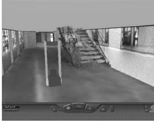
Figure 9-14. The map can be used to visualize information in 3D by augmenting with virtual content, here for example the position of the robot.
