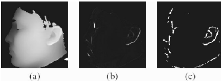
Figure 6-7. (a) Original side face range image. (b) Its step edge magnitude image. (c) Its step edge image.
