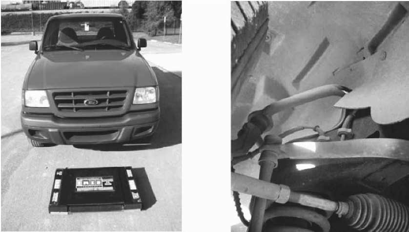
Figure 11-2. An alternative to a mirror-based inspection is a low-profile mobile robotics platform (called SafeBot) that can navigate under a vehicle while inspection personnel remain at a safe distance. On the right, we see a single frame from the camera on the robot. Due to low ground clearance of the automobile and restricted field of view of the camera on the robot, a single frame only shows a small section of the undercarriage.
